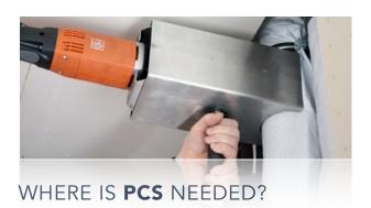
PCS was specifically designed for applying precision square cuts under restraining conditions and in virtually inaccessible locations, such as corners, shafts and when pipes run parallel without much space in between. It can be used to cut sewage and water pipes, retrofitting of diversion and T-branches or similar applications.
